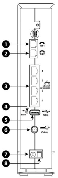
1. Connect one end of the coax cable to the cable outlet or splitter, and the other end to the Telephony Gateway's Cable connector (**6**). Tighten the connections by hand, then tighten an additional 1/8 turn with a wrench.
